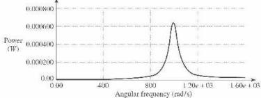
Note that as the angular frequency goes to zero, the power and current are zero, just as they are when the angular frequency goes to infinity. This graph exhibits the same strongly peaked nature as the light red curve in Fig. (31.15).
